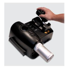
Testing and calibration with the AutoRAE Lite are simple—just cradle the instrument and press a button.
